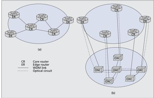
■ Figure 1. Architectures of an optical transport network employing OPS nodes: a) pure OPS; b) OPS + optical circuit network.
